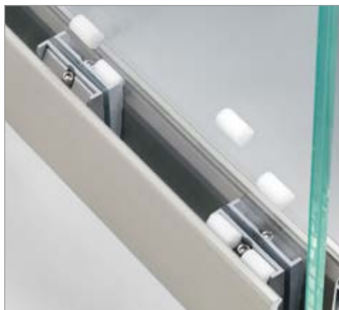
5 POM wedges insertion. The wedges ensure the best load distribution to the glass / clamp / profile interface, maximizing system performance.
