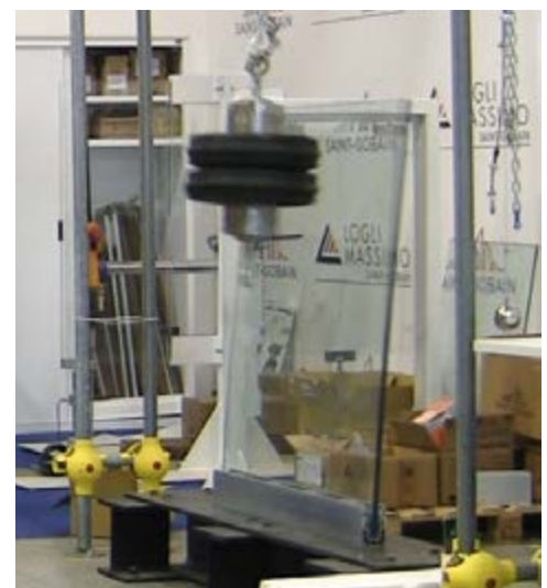
Dynamic impact test from a semi-rigid body 50 kg (EN12600) Hc = 70 cm, Hv = 110 cm
