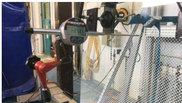
SLE static load test, 1.0 kN / m, Hs = 110 cm
