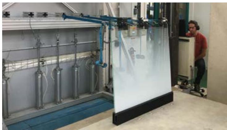
Static load test 3.0 kN / m Hs = 110 cm
