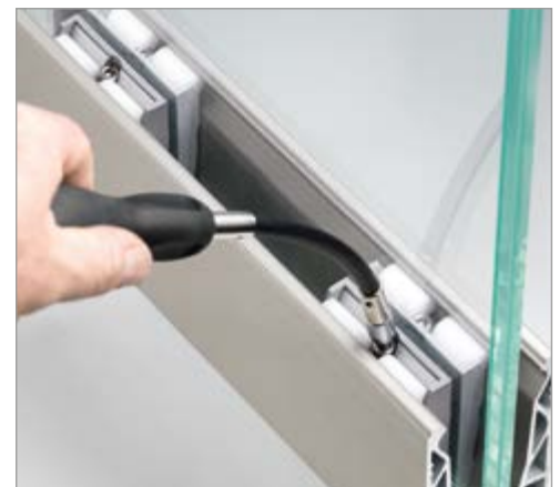
6 Adjustment from the top of the pre-installed aluminum presser, using a hexagonal head screwdriver. Maximized adjustment speed. It is possible to complete the adjustment using an automatic screwdriver. Tightening torque 3 Nm.
